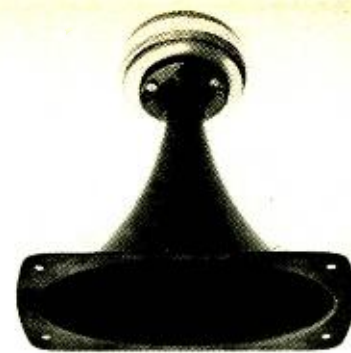
ance: 8 ohms. Flare cutoff: 1000 Hz. Magnet wt: 12-oz oriented ceramic. Size: 8 7/8" depth overall, 3 1/2" x 8" mouth. Weight: 2 1/2 lb.—Cleveland Electronics Inc., Cleveland, Ohio
