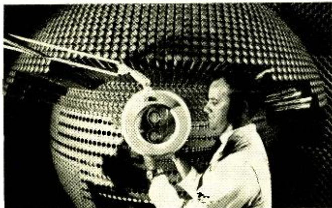
Engineer Ray Lanctot adjusts one of the many energy feeds.
