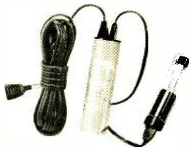
flash tube separated from the other circuitry by a 23" cord; and a small cylinder
